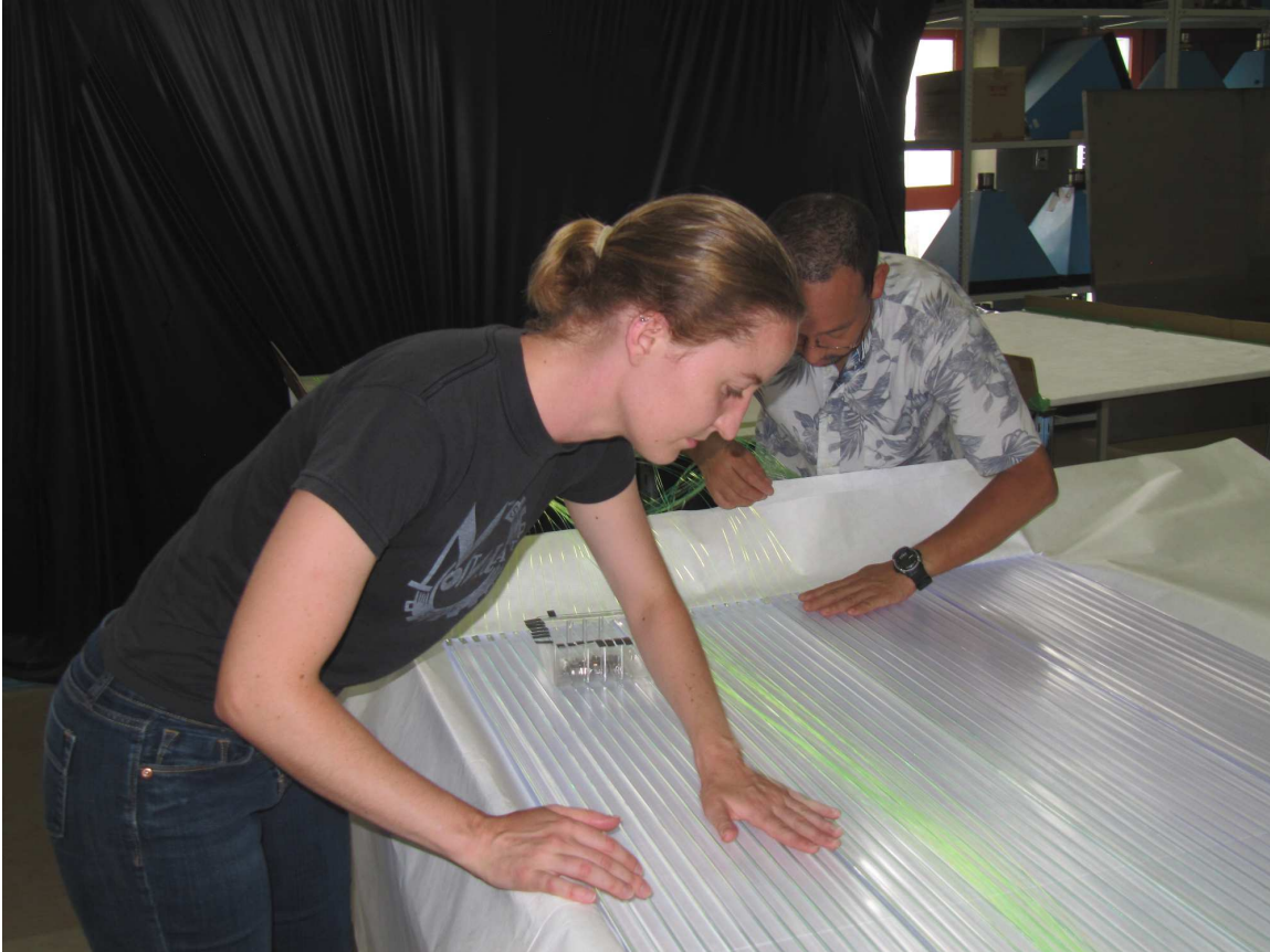
Figure 3.5. Placement of the wavelength shifting fibers in the grooves in the scintillating plastic in a SD: each fiber was individually placed by hand and taped at the two ends. Optical fibers from each layer are glued into bundles (four bundles per layer: two for each end of each piece of plastic). These are then mated with the PMTs, one per scintillator layer.
