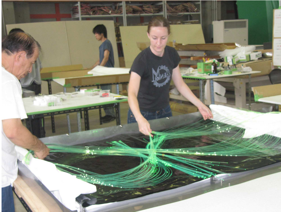
Figure 3.3. The SD construction facility at the University of Tokyo’s Akeno Observatory in Akeno, Japan: in the photo, we are preparing the wavelength shifting fibers to be attached to PMTs.
