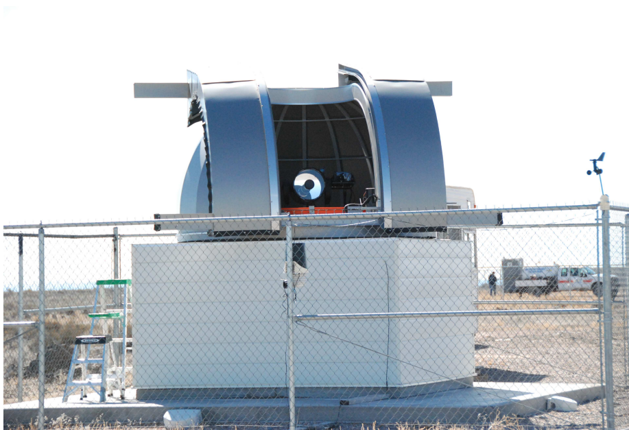
Figure 3.27. This photograph shows the monostatic LIDAR facility located at the Black Rock Mesa Fluorescence Detector (BRMFD). It houses a Nd: YAG laser used for measuring the Vertical Aerosol Optical Depth (VAOD).
