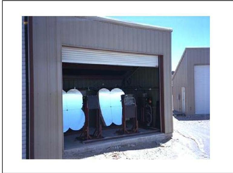
**Figure 4.1.** A picture of a detector building at the HiRes-2 observatory. Each building is approximately the size of a two-car garage. The mirrors are each made of four segments giving them a “clover leaf” appearance. The spherical mirrors are each approximately  $2m$  in size and focus the light onto the PMT camera approximately 92 inches in from the center of the mirror. An electronic rack may be seen at the far right in the building.
