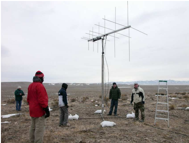
Figure 5: Radar receiver antenna at Long Ridge fluorescence detector site.
