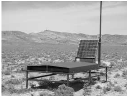
Figure 2: A picture of deployed SD. Electronics box and scintillator are on the iron frame. An electronics exists under the solar panel and scintillator box exists under the roof visible at the picture. Each SD are deployed in 1.2km of separation.
