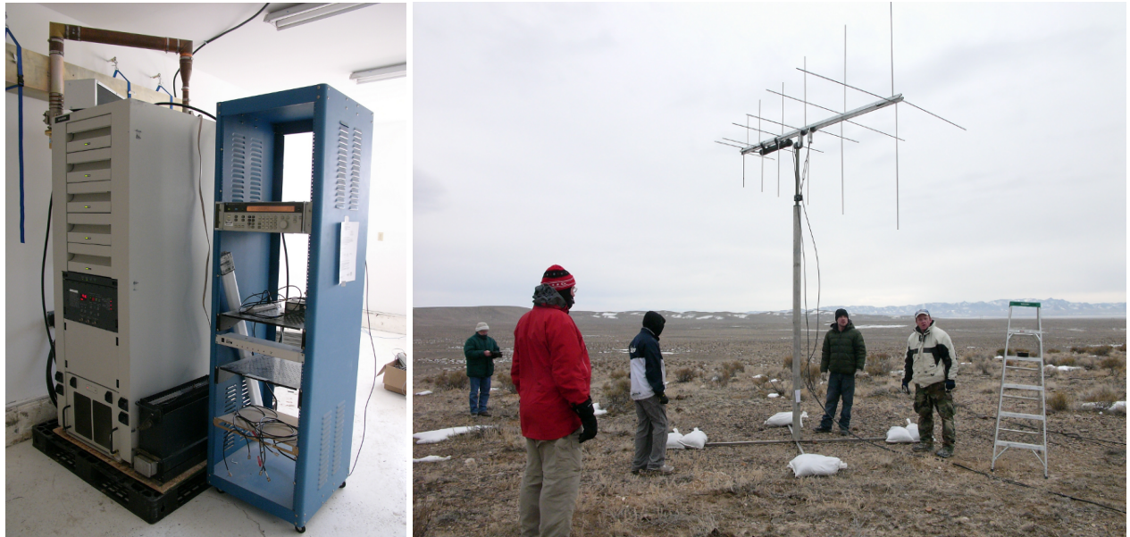
FIGURE 3. Left: 2 kW “Channel 2” transmitter donated by KUTV-2, in operation at Delta Cosmic Ray Center. Right: Radar receiver antenna at Long Ridge fluorescence detector site. First of four. (Photos: Helio Takai)
