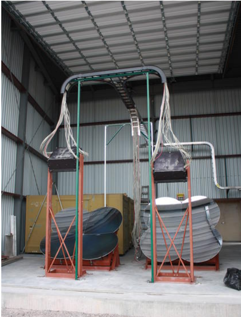
Figure 4.5: Front View of TALE Telescopes. This is an image of a pair of TALE telescopes as seen when facing the mirrors. The four-segmented lobes of each mirror are clearly seen in this photograph. Additionally, the cable tray that connects the PMT camera to the readout electronics is also visible. As can be seen, the readout cables for each pair of cameras in a garage bay are bundled together.
