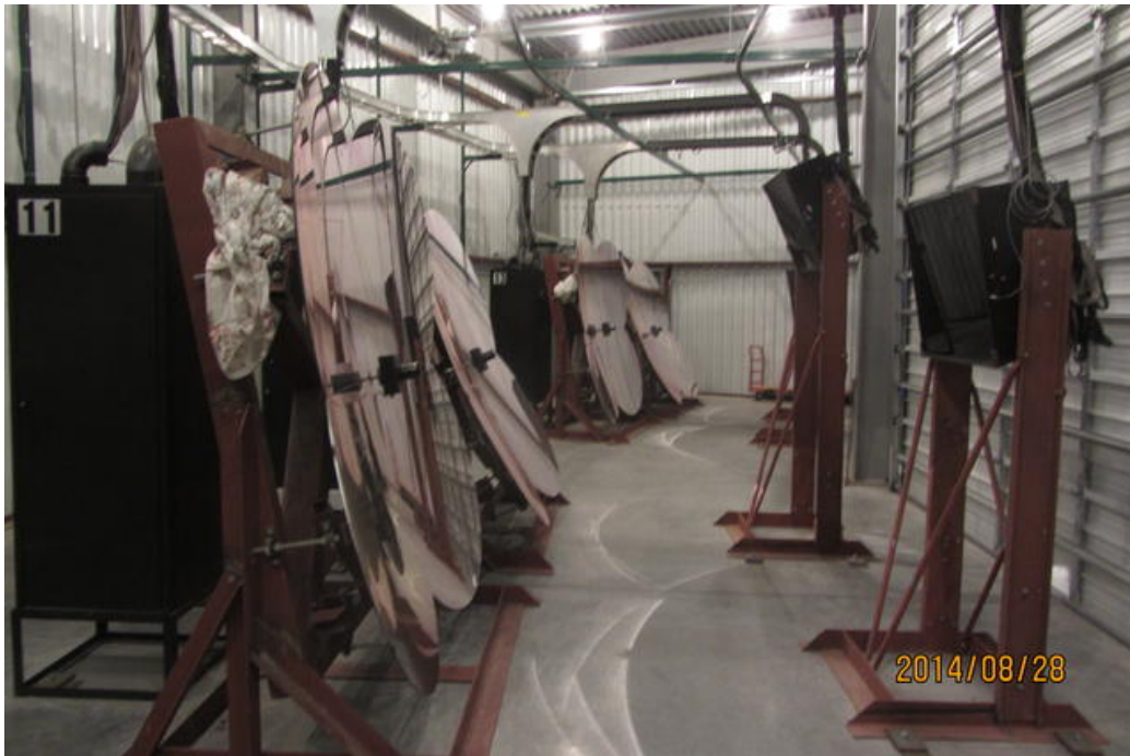
Figure 2.11: Photograph of Telescopes at the MD Station. A telescope consists of a clover leaf spherical mirror which is used to gather fluorescence light generated by EASs and focus it onto a camera consisting of a cluster of PMTs. The cluster of PMTs can be seen to the right of the mirror although a UV filter placed in front of the PMTs prevents seeing the honeycomb pattern the PMTs are arranged in. Behind the mirror is the electronics crate responsible for triggering on and reading out the PMT signals.
