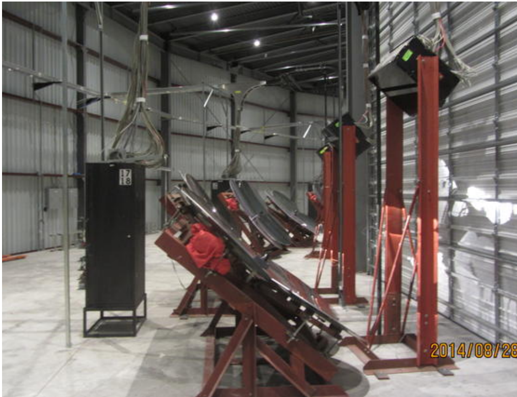
Figure 4.3: Side View of TALE Telescope. The spherical mirror is in the center of the image and is used to focus light from CR air showers onto the PMT camera box mounted on the red stand to the right of the image. The readout electronics for a pair of cameras are housed in the black rack on the left of the image labeled 17,18.
