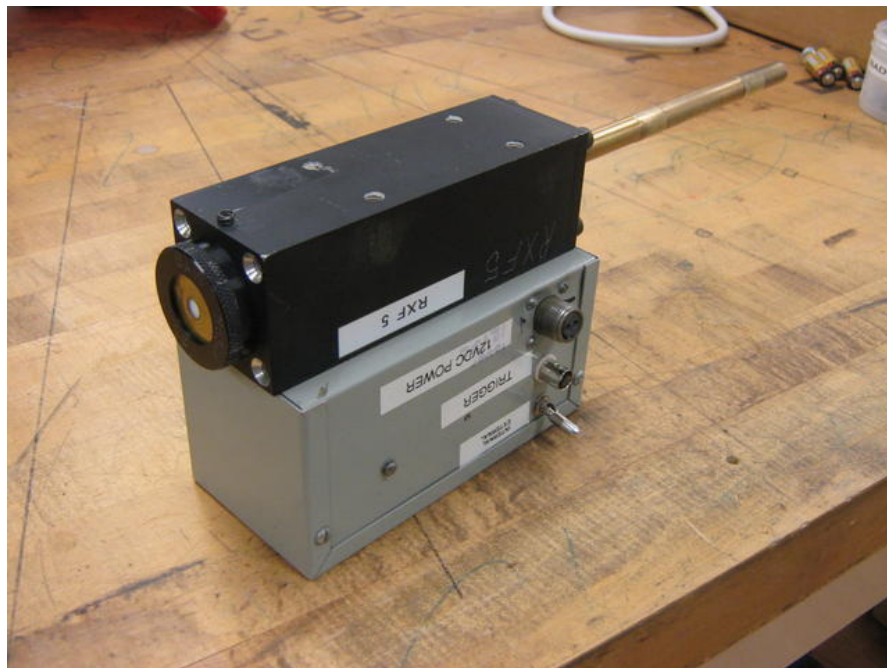
Figure 2.11: Photo of the RXF module. The black box contains the Xenon flash lamp itself. The black cylinder at the front of the RXF contains the optical filters (band pass and narrow band) as well as the teflon diffuser, and a brass aperture. at the rear of the black box is a 1/2" brass rod that is used to mount the RXF in the center of post. The grey box below the black box contains the electronics for charging and firing the RXF flash lamp. Reprinted with permission from J. N. Matthews.
