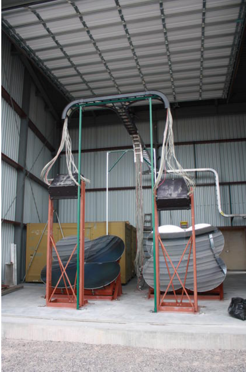
Figure 2.14: A pair of TALE telescopes with viewing angle of 30^{\circ} - 59^{\circ} in elevation. From the photo, it is apparent that these telescopes are tilted up significantly as compared with the MD telescopes. Reprinted with permission from J. N. Matthews.
