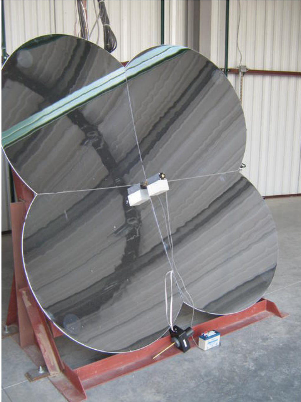
Figure 2.12: Photo of RXF placed at the center of the mirror. At the bottom of the mirror, one can see the 12 V battery (grey and blue colored box) that is providing power to the RXF and the UVLED, which is normally mounted in the center post and provides a nightly relative calibration. Reprinted with permission from J. N. Matthews.
