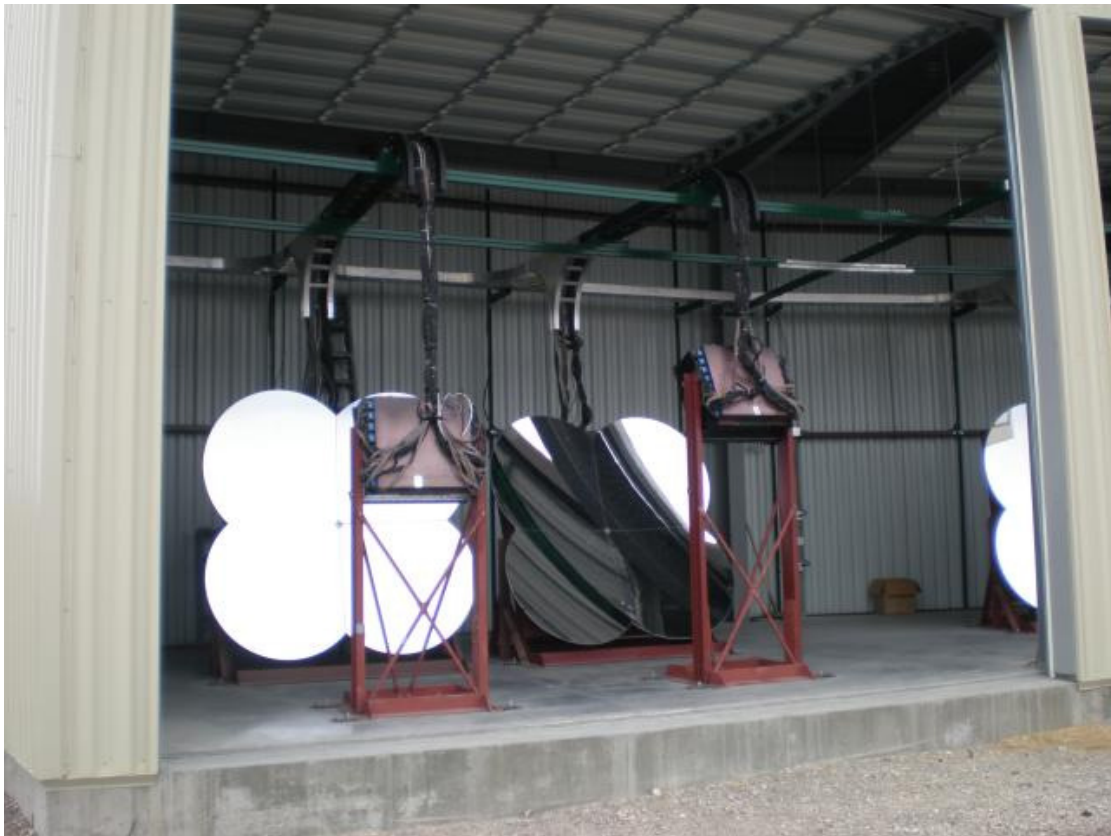
Figure 2.4: A pair of MD telescopes covering viewing angle of 3^{\circ} - 31^{\circ} in elevation. Reprinted with permission from J. N. Matthews.
