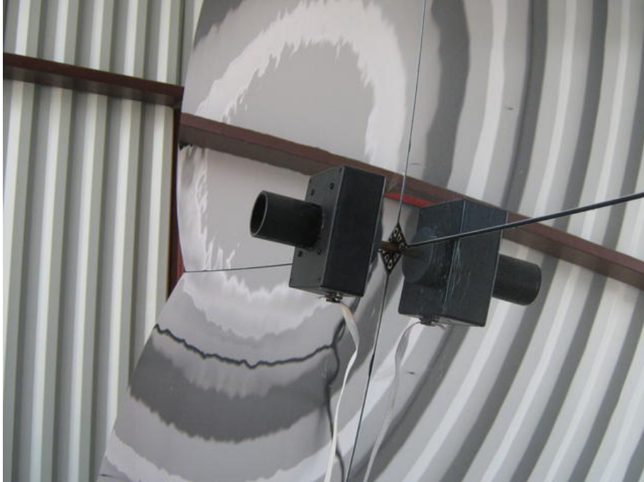
Figure 2.21: Photo of UVLED module placed at the center of a mirror. Reprinted with permission from J. N. Matthews.
