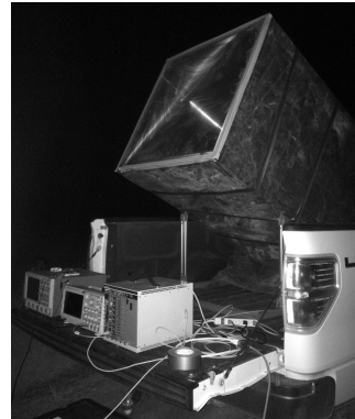
Figure 6: Photo of CRAFFT telescope operating from the bed of a pickup truck.
