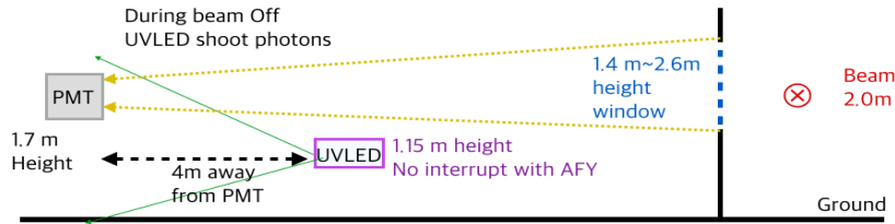
Figure 3. On site calibration using UVLED, The calibration was operated when beam off. The UVLED was position at lower than a path of AFY, so it was not interrupt with AFY measurement.
