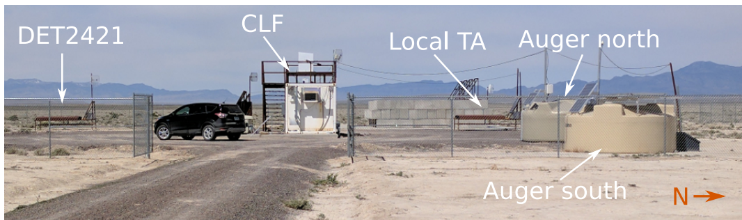
Figure 1: Photo of hardware deployed at the TA CLF site. Custom cabling was setup along guy wires from stations to the CLF for data acquisition. North is to the right of the page.
