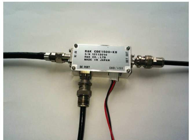
Fig. 3. Electric-circuit unit R&K CDE1500-KU developed with the R&K Company. A bias-T, impedance converter, and power detector are packed into a compact case.
