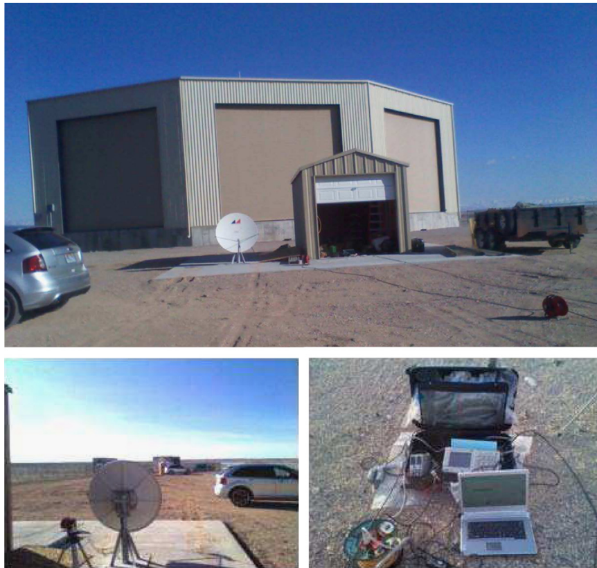
Fig. 5. Photographs of the observation system installed at the TA observatory. The upper panel shows the parabola located in front of the FD building. The lower-left panel shows the parabola as seen from behind. The ELS is visible 85 m away from the parabola. The lower-right panel shows the data-acquisition system. The entire system is packed into a suitcase that can be transferred by commercial air flight from the laboratory to the observation site.
