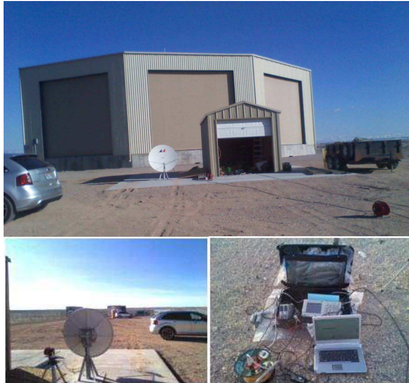
Figure 3: Photographs of the observation system installed at TA observatory. The upper panel shows the parabola located in front of the FD building. The lower-left panel shows the parabola seen from behind. The ELS is visible 88 m away from the parabola. The lower-right panel shows the data-acquisition system. The entire system is packed in a suitcase so that it may be transferred by commercial air travel from the laboratory to the observation site.
