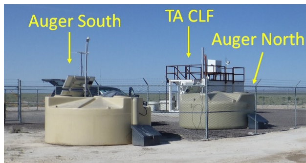
Figure 1: The two Auger SD stations deployed at the TA Central Laser Facility.
