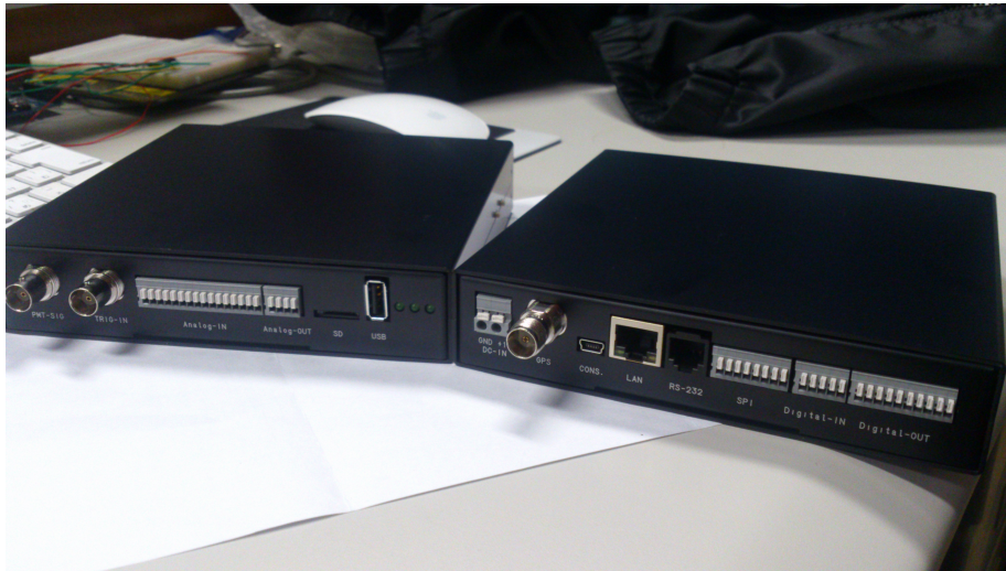
Figure 3: The front and back of the data acquisition models from Brains, Inc.
