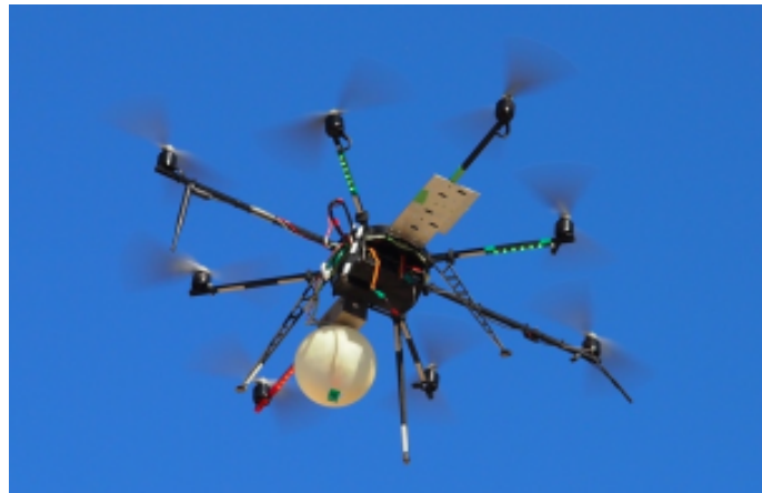
Figure 3: Octocopter : a radio-controlled helicopter with 8 rotors. At the bottom of the octocopter, the LED flasher is mounted.
