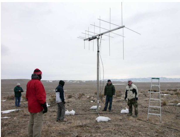
Fig. 3: Radar receiver antenna at Long Ridge fluorescence detector site.
