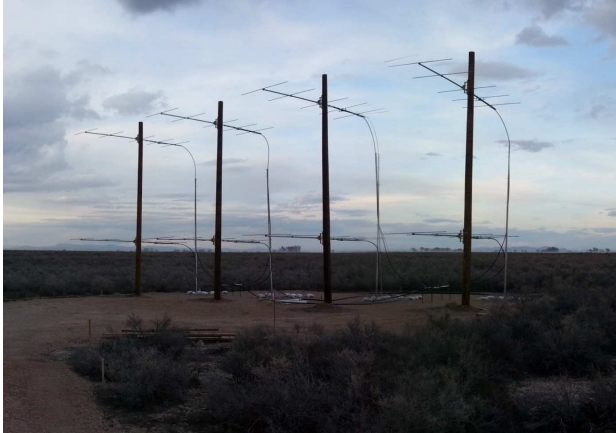
Fig. 5: Phased array of 8 Yagi antennas, increasing transmitter gain to a factor of 21 dB over isotropic.
